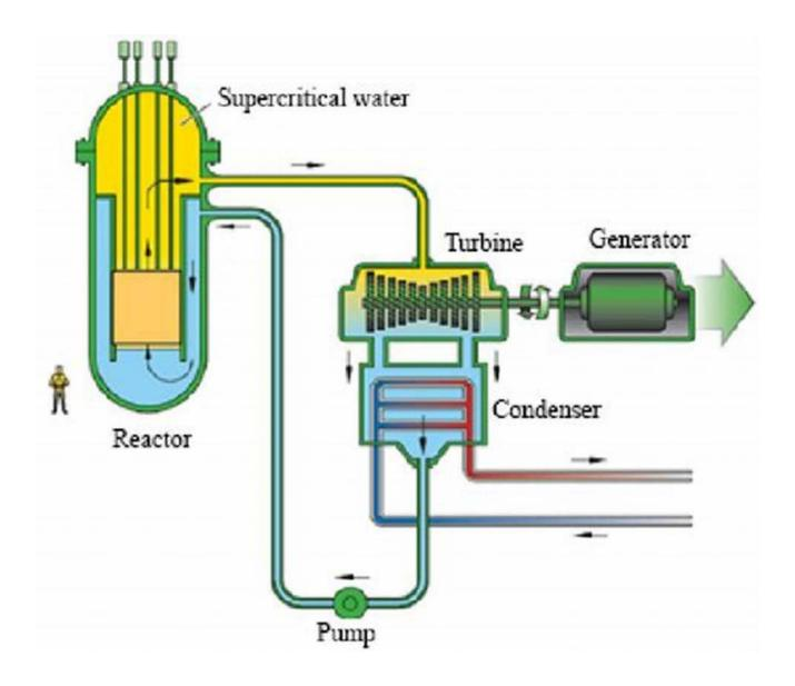
Supercritical Water Cooled Reactors (SCWRs) have gained significant attention in recent years due to their potential as a sustainable and efficient source of nuclear energy. With the aim of improving safety, efficiency, and reducing waste, researchers and engineers have focused on understanding the behavior of materials and the importance of water chemistry within these advanced reactor systems.
