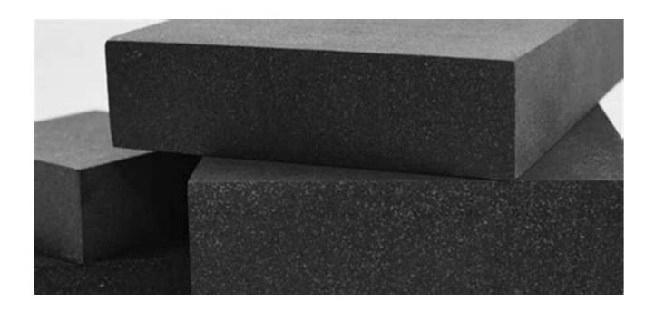
Carbon foam, crafted from a three-dimensional network of carbon atoms, combines low density with exceptional thermal insulation properties. Its lightweight nature, excellent heat resistance, and unique structure make it an invaluable material in aerospace, automotive, and renewable energy industries. Carbon foam has the potential to revolutionize how we insulate and conserve energy.
