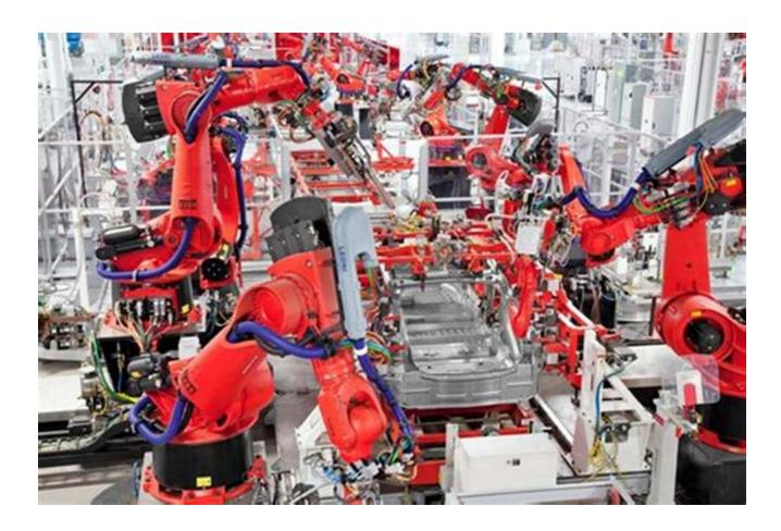
Fourth-grade children will be fascinated to learn about the role of robots in the manufacturing process. They can explore how these machines handle welding, painting, and assembly operations with precision and speed that surpass human
